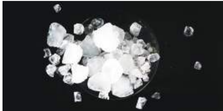
Aluminium Sulphate from Waste Dross
