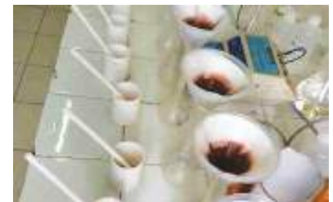
Selective enrichment of \text{Fe}_2\text{O}_3 in red mud
