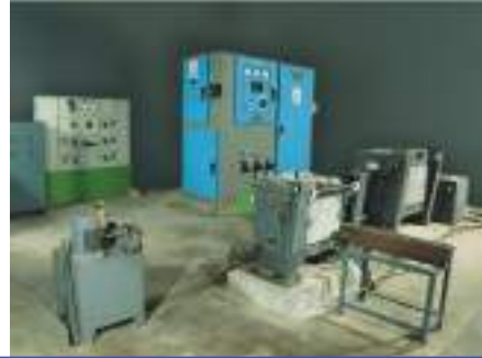
Induction Melting Furnace
