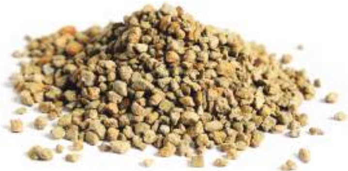
Refractory Aggregates from Saproliite
