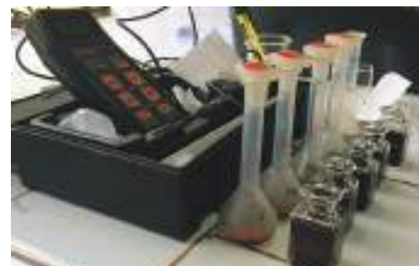
Colourimetric analysis of Ca in hydrate, alumina & liquor
