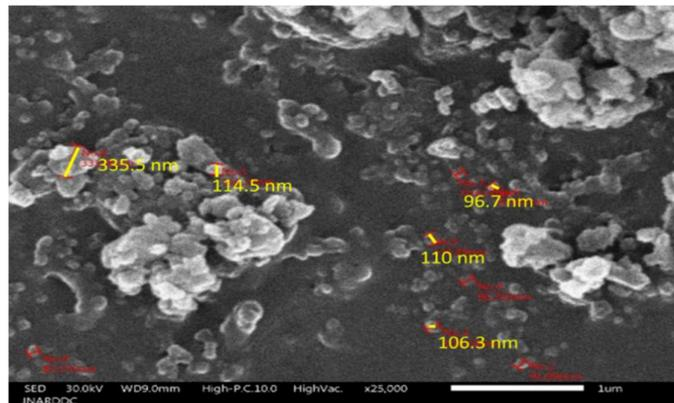
Microstructure of nano-size ATH in Scanning Electron Microscope
